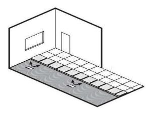
Tip over a row of tiles at a time. Spread the adhesive with the proper not chedrowel as advised by the manufacturer.
