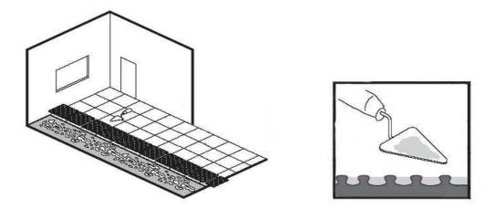
Tip over the first row of tiles. Fill properly the dove-tail backing of the tiles with amixture of 325 cement, sand (ratio 2:1) and water to obtain a suitable density.
