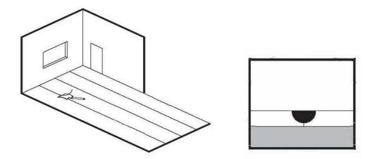
When the rod has cooled to room temperature the remaining excess should be trimmed using the spatula knife without the guide keeping a shallow angle between blade and floor to avoid "digging in". Attention: the colour of the rod cannot be exactly the same of the floor.
