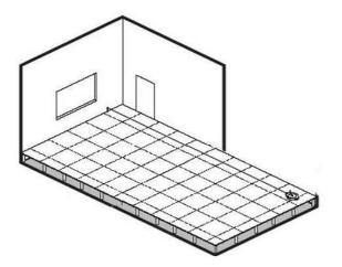
Measure the room and mark the centrelines planning the laying in a way to reduce cuts and scraps.
