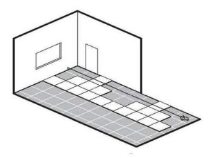
Measure the room and mark the centrelines planning the laying in a way to reduce cuts and scraps.
