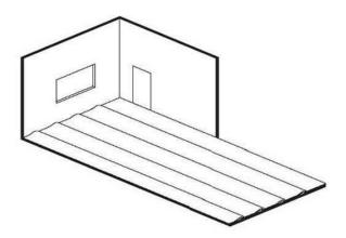
The loose laying is very important to check the colour uniformity and the absence of defects of the flooring. All claims will be accepted only if the flooring is not yet permanently bonded.
